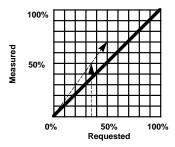
Figure 5 - When a requested 50% halftone dot becomes 70% because of dot gain, a 36% requested dot actually results in a 50% measured halftone dot.
