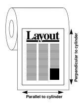
Figure 2 - The distortion of a photopolymer flexographic plate occurs perpendicular to the shaft of the printing cylinder.
