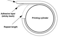
Figure 3 - Cross section of a flexographic printing cylinder showing the variables involved in distortion.
