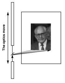
Figure 2 - With a drum device the optical system moves, often on a spindle as shown here. The film is attached either to the inside or outside of the drum.
