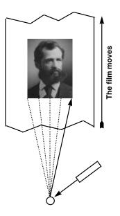
Figure 1 - With a capstan device, the optical system remains stationary, and passes a laser beam across a moving piece of film.
